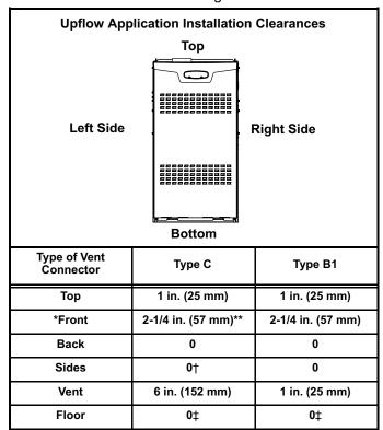
\*Front clearance in alcove installation must be 24 in. (610 mm). Maintain a minimum of 24 in. (610 mm) for front service access. \*\* 4-1/2" if single wall vent pipe is used.
